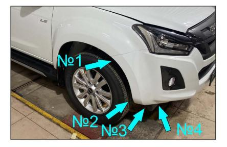
7. Unscrew all fastening elements on **each** bumper sides (see step 8 – step 11).
