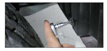
9. Unscrew the screw which attaches mudguard to bracket (see step 7 No. 2).
