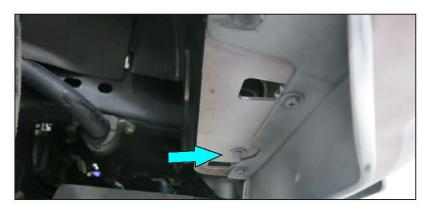
10. Unscrew the nut which attaches mudguard to bumper (see step 7 No. 3).
