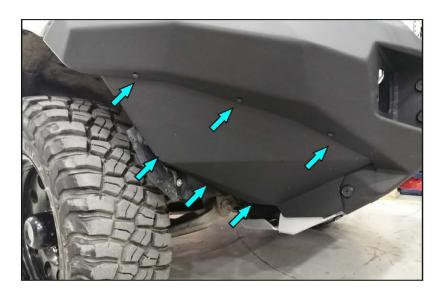
29. Install flaps (pos. 4, 5) on aluminum bumper body using M6x20 screws (pos. D) and washers 6 (pos. J), tightly press the flaps and mark cutting line and holes for drilling.
