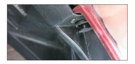
8. Remove plastic eyelets which attach mudguard to bumper (see step 7 No. 1).
