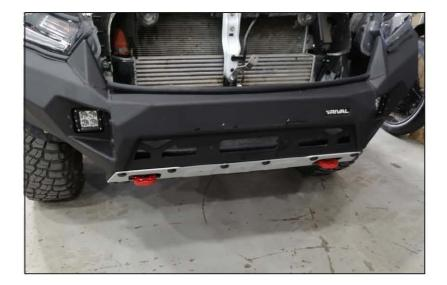
25. Adjust bumper until you have an equal gap between vehicle body and the bumper on both sides. Tighten bolts after that.
