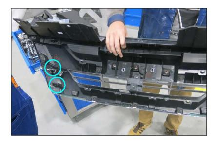
5. Remove radiator grille by detaching 2 latches from bumper on each side
