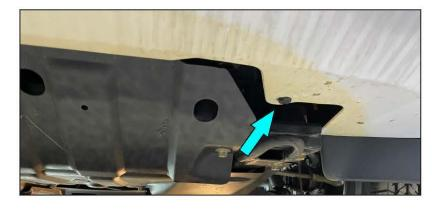
11. Remove plastic eyelets which attach mudguard to bumper (see step 7 No. 4).
